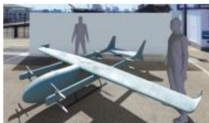
Figure 1. A render of a Mugin-5 Pro, 5m wing-span VTOL fixed-wing drone, with human for scale, capable of carrying industry approved packages.
